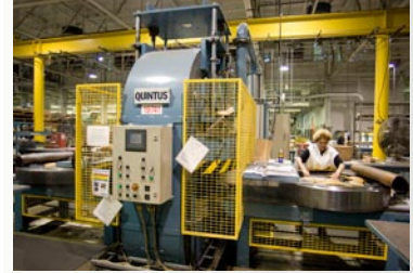
Cessna's two Flexform presses each feature Quintus™ wire-wound technology to reinforce the pressure vessel and frame.
