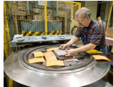
The Model QFL precisely forms multiple parts in a single 1.3 minute cycle.
