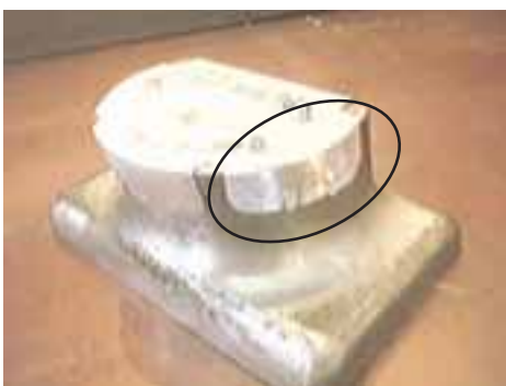
Figure 1. Typical example of tooling used with lower pressure rubber pad presses
