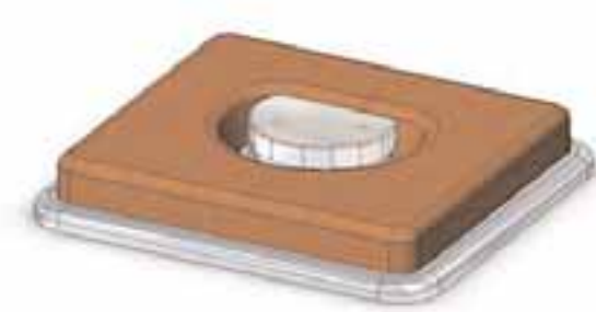
Figure 3. Redesigned Flexform tool with blank holder
