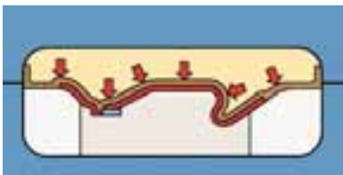
Oil under very high pressure forces the rubber diaphragm to wrap the blank completely and uniformly around the tool half.
