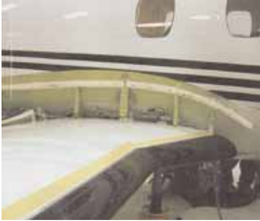
Figure 5. Eclipse wing-to-body fairing attachment
